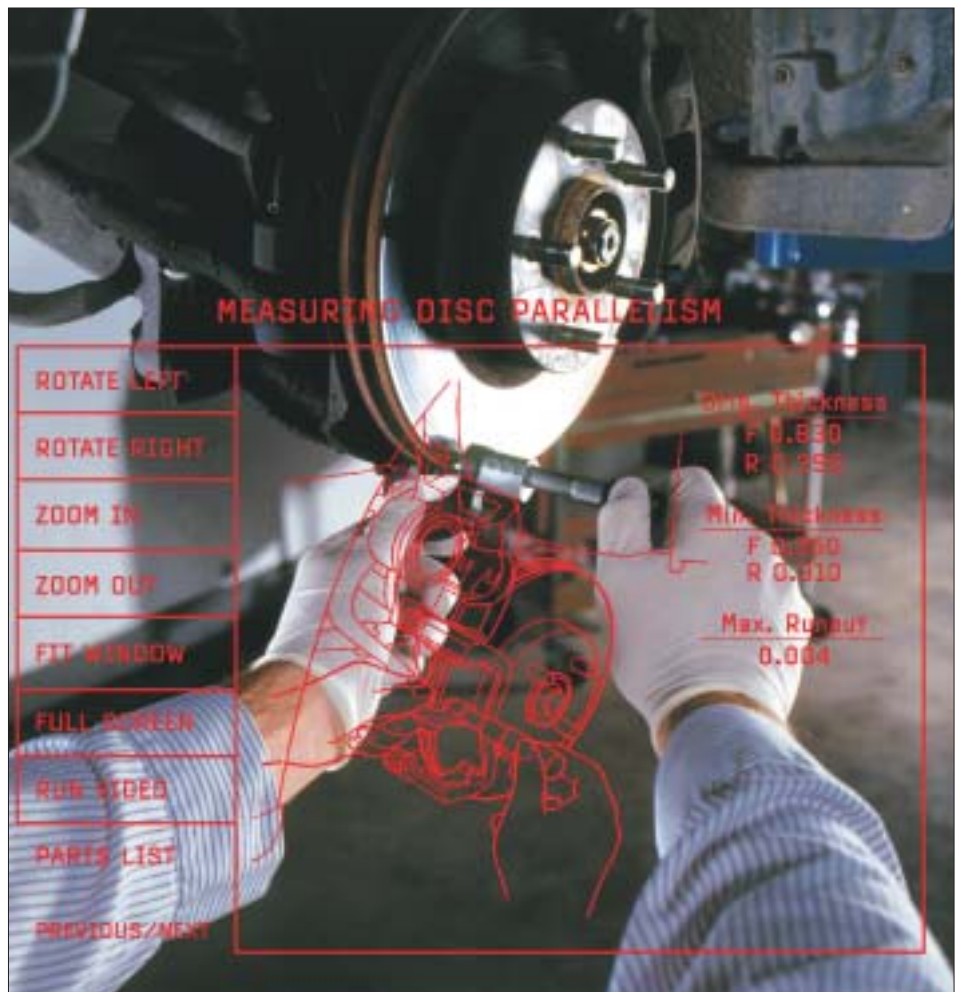
The 18-ounce Nomad System uses a MEMS device to superimpose high-contrast, high-resolution images on its user's view of the surrounding environment. Photo: Microvision
