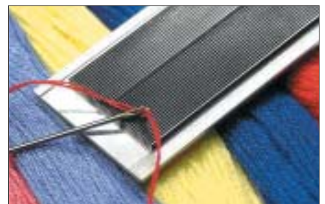
Because they produce very high rates of heat and mass transfer, microchannels 10-100 microns thick are the key to a number of technologies being developed by the Microproducts Breakthrough Institute. Photo: PNNL
